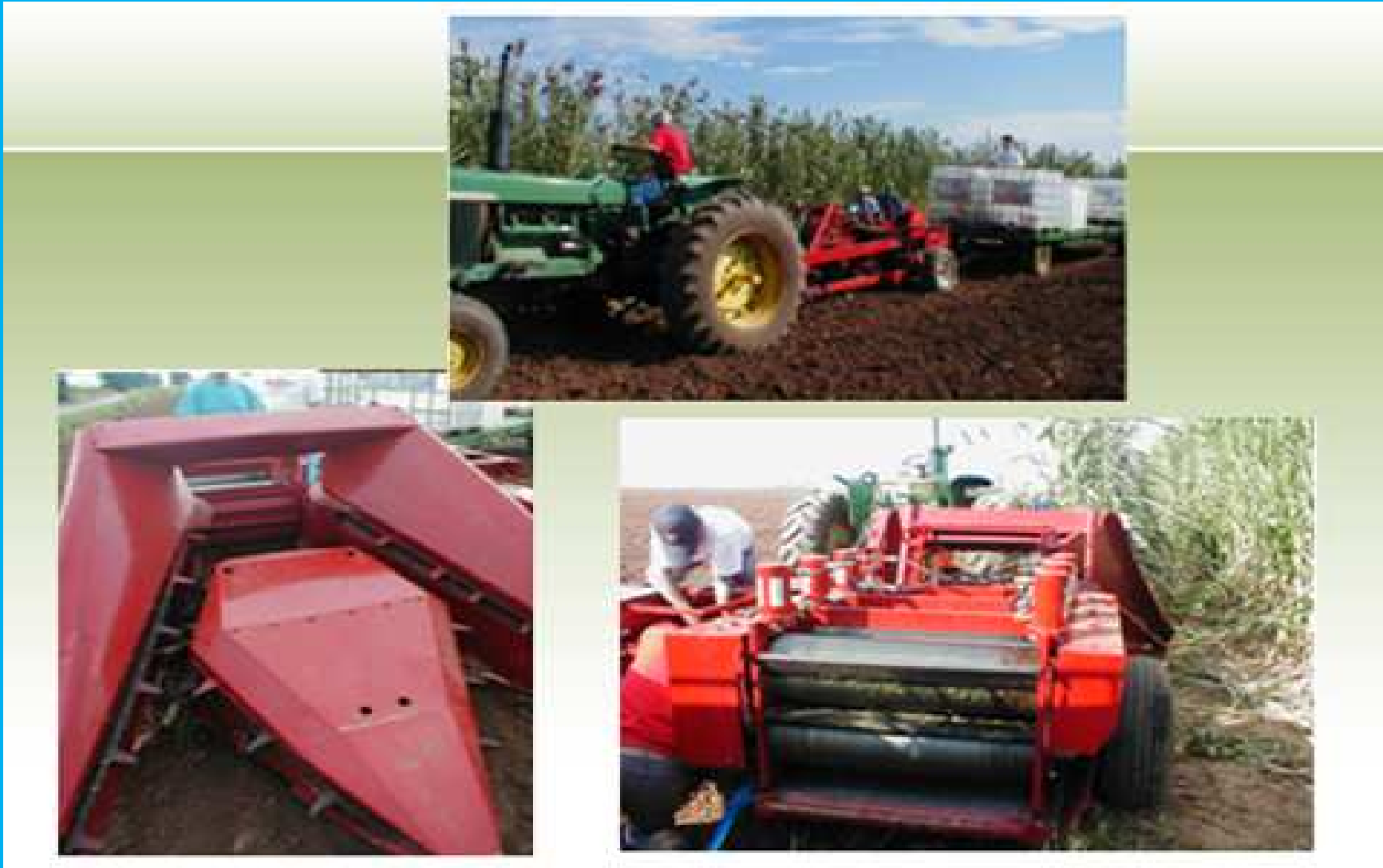
Fig. 15. Sweet sorghum Harvesting and Jus extraction in the same pass using the Mc Cluny Sor-cane Harvester in large farms..(photo: Mc Cluny Industries) [10]
